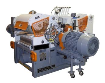
The Newman EPR Electric Series Double Roughing Planers provide state-of-the-art technology backed by the world's most experienced planer manufacturer. Newman's new EPR Series Planers feature electric feed drive. Additional innovative features include an improved locking mechanism for the cutterhead leveling system and redesigned bottom cutterhead dust collection.
